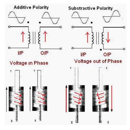
When Pair of Coil of Transformer have same direction than voltage induced in both coil are in same direction from one end to other end. When two coil have opposite winding direction than Voltage induced in both coil are in opposite direction.
